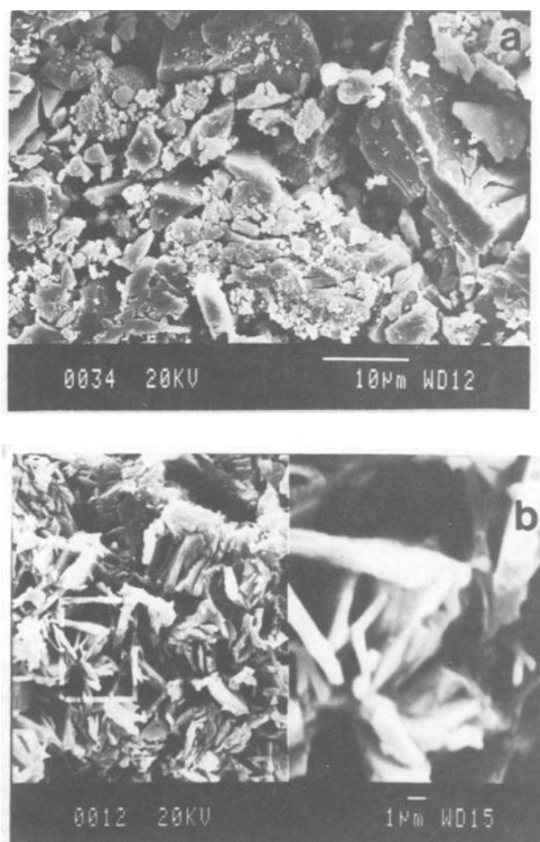
Fig. 2. Scanning electron micrographs of samples: a) 0.5\text{La}_2\text{O}_3 , 0.5\text{Y}_2\text{O}_3 ; b) 0.8\text{La}_2\text{O}_3 , 0.2\text{Y}_2\text{O}_3 .
